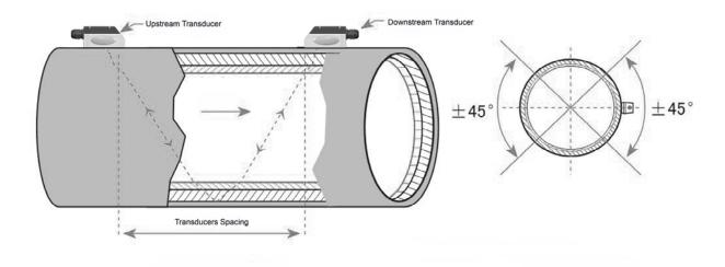
V-method installation is the most widely mode for daily measurement with pipe inner diameters ranging from 15 mm to 200 mm. It is also called reflective mode.
